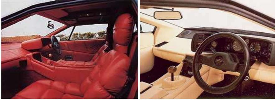
Cockpit changes have been made, including an instrument panel which now boasts a turbo boost gauge and speedometer running up to 170mph. Air conditioning controls are now situated in a centre console panel and all switchgear is backlit when main and side lights are illuminated. The seats have revised foam foundations and with new head restraints.
