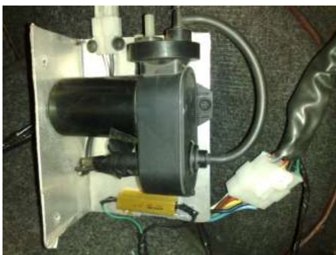
Picture showing the position of the resistor and the 8 pin connector for reference
