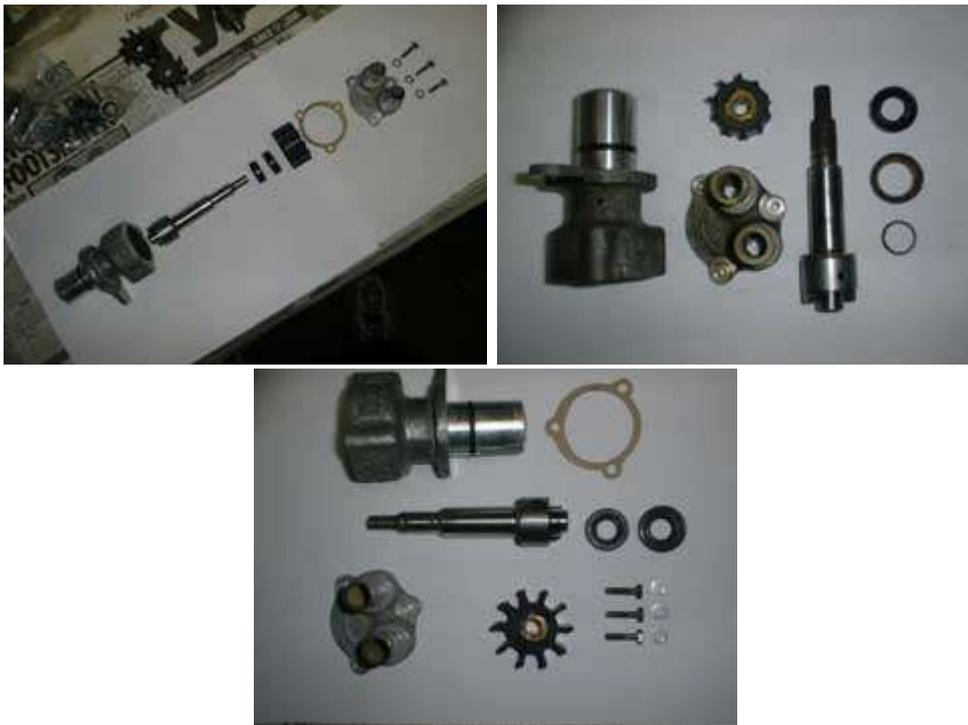
5 . Clean the mating faces of the pump body and end cover, removing ail traces of the old gasket, and ensure that the inside of the housing is thoroughly cleaned. Smear some petroleum jelly around the inside of the pump housing and on the shaft.
