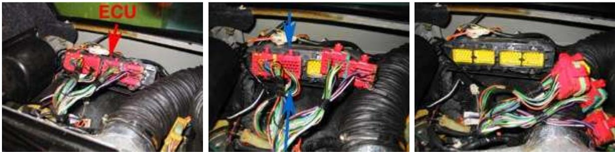
You'll see the ECU as soon as the covers removed. It's the black box with four large red connectors attached to it. You now need to remove the wires from the ECU. Push down top and bottom of each connector and pull them off. Mine were a little stiff and needed pushing down quite hard. (If you don't want to disconnect the ECU, you can turn it over and remove the chip while it's still attached). Remember to note which connector is attached in which order. This will help when replacing the ECU.
