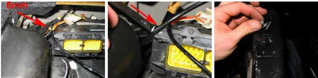
The ECU is held into the Esprit by two 8mm nuts. Space is at a minimum, so you'll find it difficult to get a socket in. I used a spanner and could only get a quarter turn on it. So it took a while to undo! Be careful not to lose the nut once it's off. As I don't think these are readily available. The thread is on a small backing plate, which slides into the ECU.
