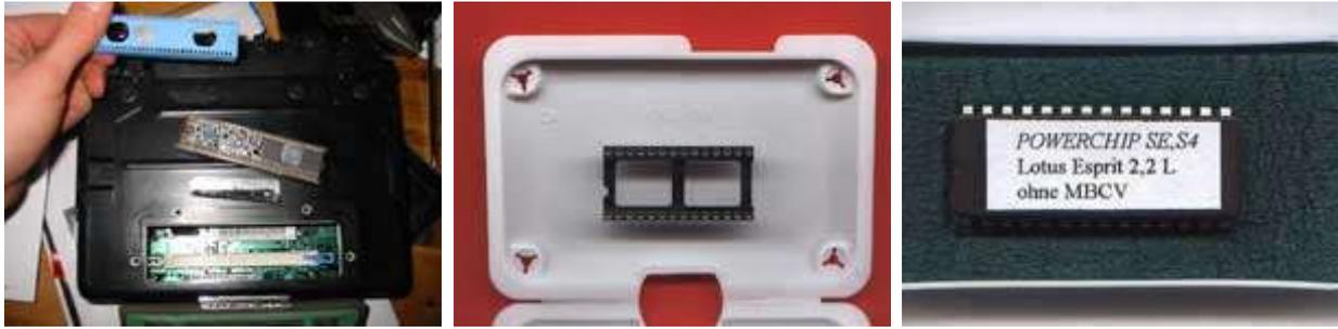
Your new chip is supplied with a chip holder. This is what will replace the chip, this will then allow you to change the chips. Now if you're happy to do the soldering yourself, take a pair of scissors and carefully cut the 28 connectors holding the chip in. You can then solder the holder into the space where the chips just been removed from.
