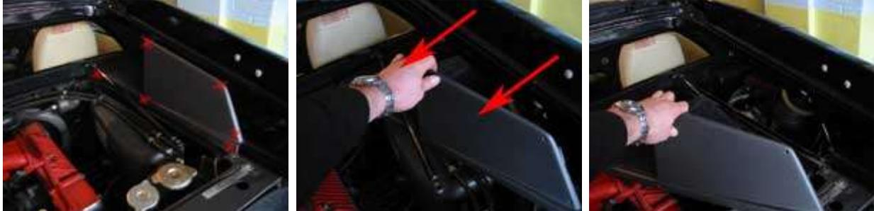
To change the chip, you'll need to take the Esprit's computer (ECU) out of the car. The ECU is located in the engine compartment, on the left-hand side, behind the airfilter (4-cylinder Esprits). It's easier to sit in the rear of the Esprit, to reach the six screws that hold the cover in place. Remove these screws and carefully pull out the cover.
