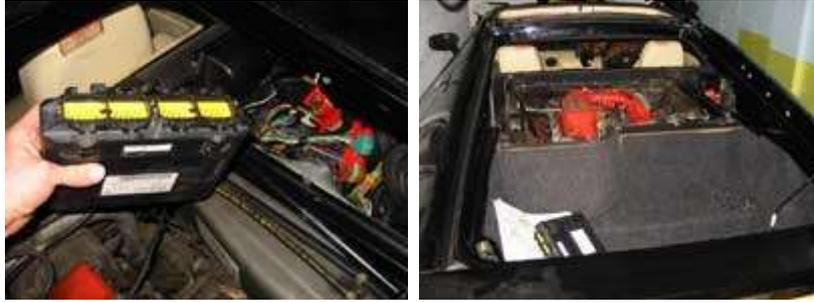
The ECU is easily removable once these nuts are removed. You can now take your ECU from the Esprit and somewhere safer than your garage to remove the chip.
