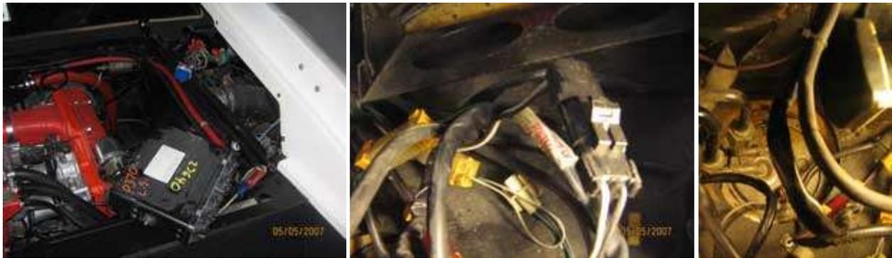
2. Remove the Right hand side (looking at the car from the rear) engine trim panel that covers the ECM. Disconnect the ECM and move it out of the way. You'll need to loosen the 8mm nuts that secure the ECM to the cradle.
