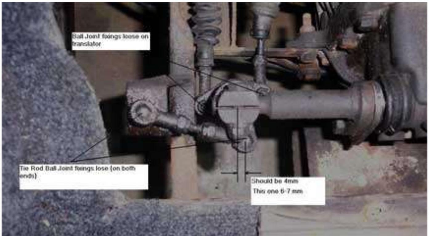
4. If necessary, adjust the length of the two cables at their rear end ball joints so that they can be connected to the translocator without preload. Note that both gearchange cables are identical and that the right hand cable at the gearlever end is fitted to the left hand side of the gearbox end. As a check, move the gear lever across the gate from right to left and observe cable movement at the rear end. The cable that moves forward is fitted to the left hand side at the gearbox.
