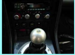
The tire pressure system looks very aftermarket (smarttire) and is not intergrated into the interior at all. Should be easily fitted to any Esprit. The alloy heater knobs (above left) aren't pre-drilled with the correct size holes for earlier Esprits. So drilling is required to retro fit.
