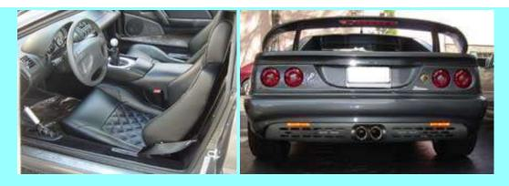
The seats have also been modified, with a new pattern stitched in. Not a worthwhile mod in my humble opinion. Lotus have also modified the infill panel around the twin center exhaust (different holes).
