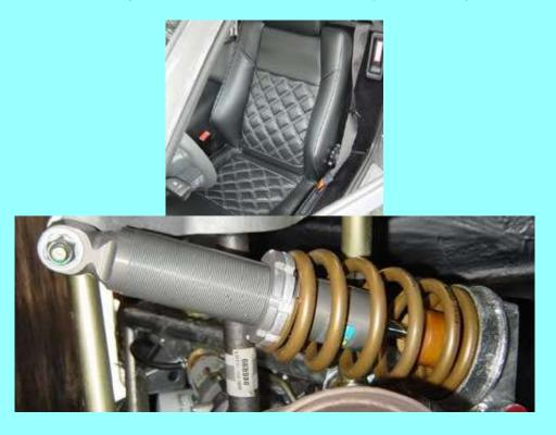
The suspension is now adjustable in height and made by eibach who are a well respected suspension manufacturer. fitted Part numbers These be easily V8's. can to all Front AO82C4257F springs х2 Rear springs AO82D4185F х2 damper AO82C4258F x2 Front Rear damper - AO82D4186F - x2
