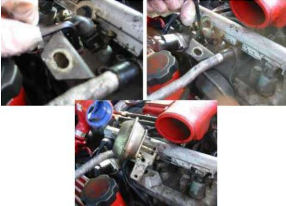
Two allen head bolts hold on the bracket, which is actually one of the chargecooler mountings. Once this is removed you can pull it and the capsule out.
