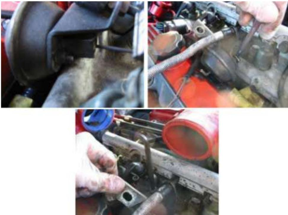
Time to remove the capsule. It's attached to a bracket with two small nuts. You need to remove the bracket to get a the nuts to release the capsule.
