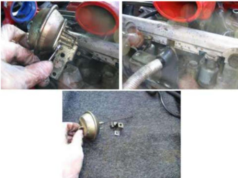
Using a small spanner you can remove the nuts and remove the capsule from the mounting. You can then replace the mounting, as the chargecooler will need it. The picture above right shows the capsule and it's fixings.
