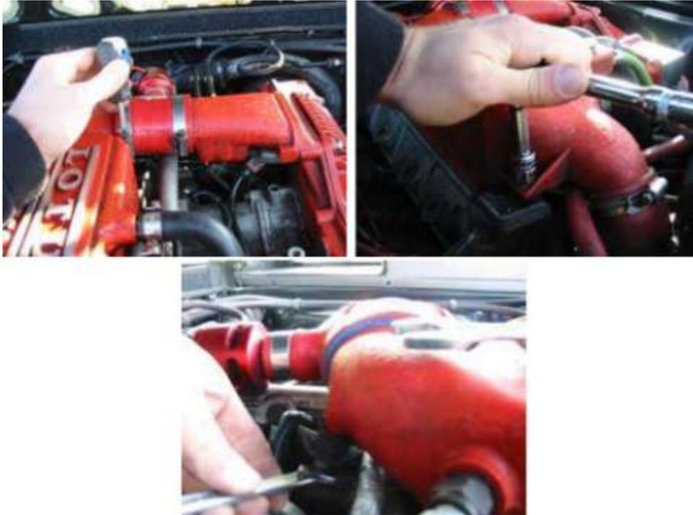
For access to the capsule, you need to remove the chargecooler. This requires the removal of 3 jubilee clips and two bolts. A full guide to removing the chargecooler can be found [here](#).
