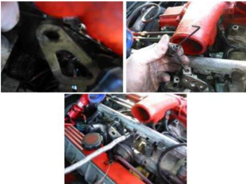
You can then remove the connection and the rod will be free. You can see the allen key in the grub in the middle picture above.
