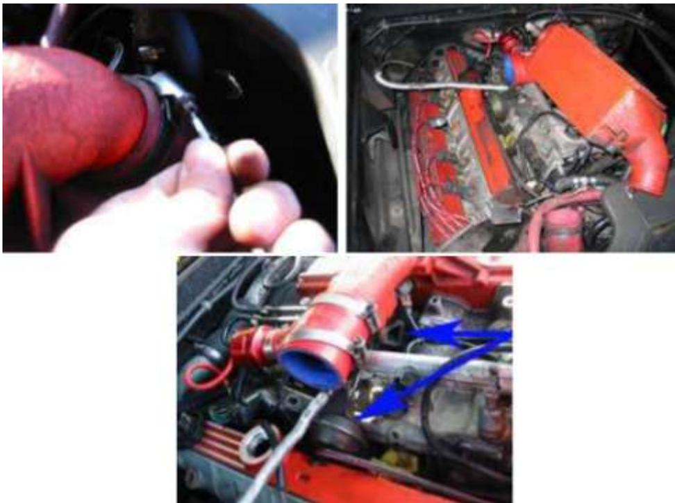
Once the chargecoolers been moved out of the way, you'll see the capsule and where the rod attaches to the throttle cable. The blue arrows point out the capsule and connection.
