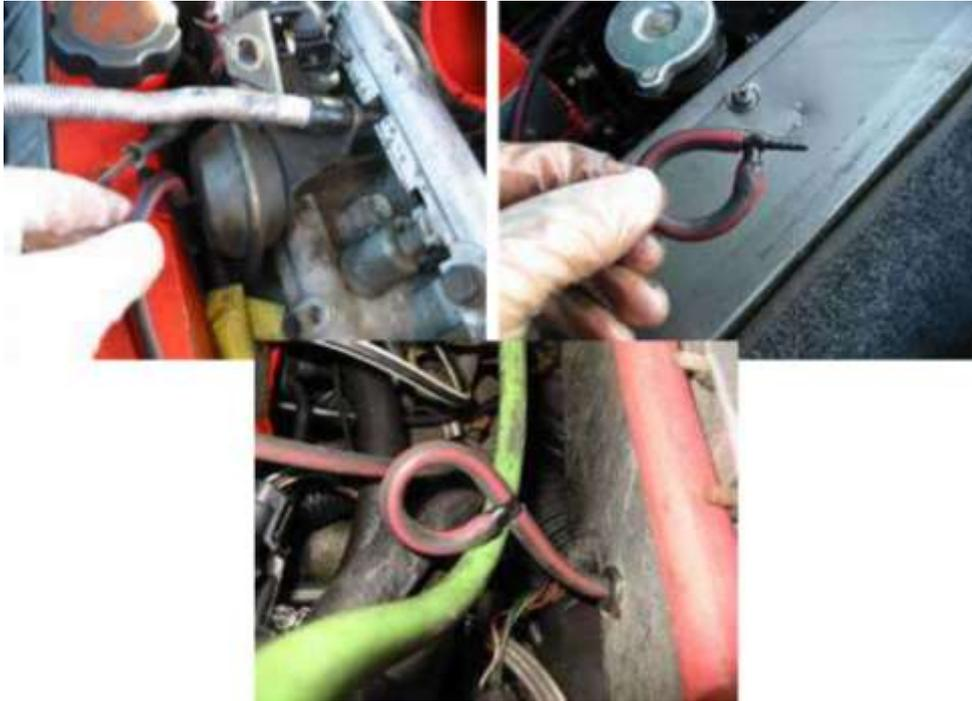
Now you need to remove the vacuum pipe from the capsule and block it off. We like to use a t-piece to feed the pipe back on it's self, We cut the pipe closer to the bodywork to keep it tidy. You can push a ball bearing into the pipe or a screw, but you must block off the pipe.
