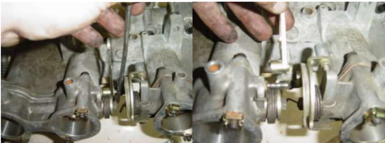
LEA has removed the quadrant successfully, you look closely of its base, the quadrant uses a clip which can be removed with a screwdriver by taking the clip away from the assembly the quadrant can be now slide from the little rod holding it, see photos below. This removal was done after we removed the inlet manifold so it was easier to access however this can be done by removing the plenum nozzle.
