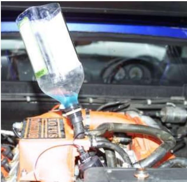
Remove both large hoses from the charge-cooler and blow through one of them to empty it. Refit the hoses.
