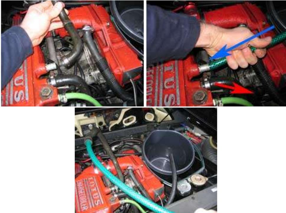
Now to flush the system, refill with some anti-freeze and bleed before putting everything back together. You should have pipe ends that were taken off the old pump. One goes to the chargecooler carrying cold water from the pump, the other comes from the radiators via the chargecooler. You can flush the system by attaching a garden hose to one end and putting the other in a bucket. Turning on the hose will flush the system out. You only needed a flow of water, so don't go turning the tap full on!
