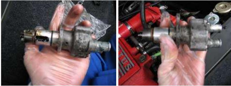
Once the bolt is removed, you should be able to pull the old pump straight out. Ours was stiff and needed some encouragement. You can now see the old mechanical pump along side its electrical replacement with the plug and bracket to fill the hole left behind.
