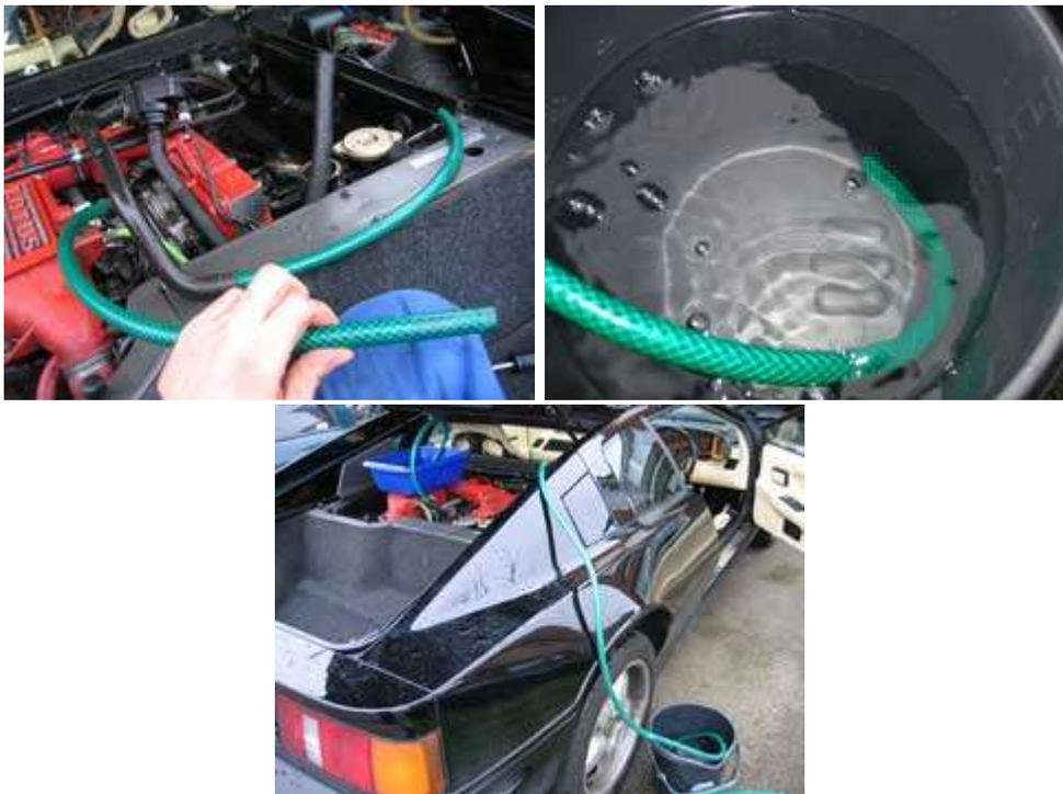
The pump was then fitted and we primed the system with clean water from the hose (no airlocks of course). Then using small plastic bucket fitted as low as poss. and a length of hose to connect to the
