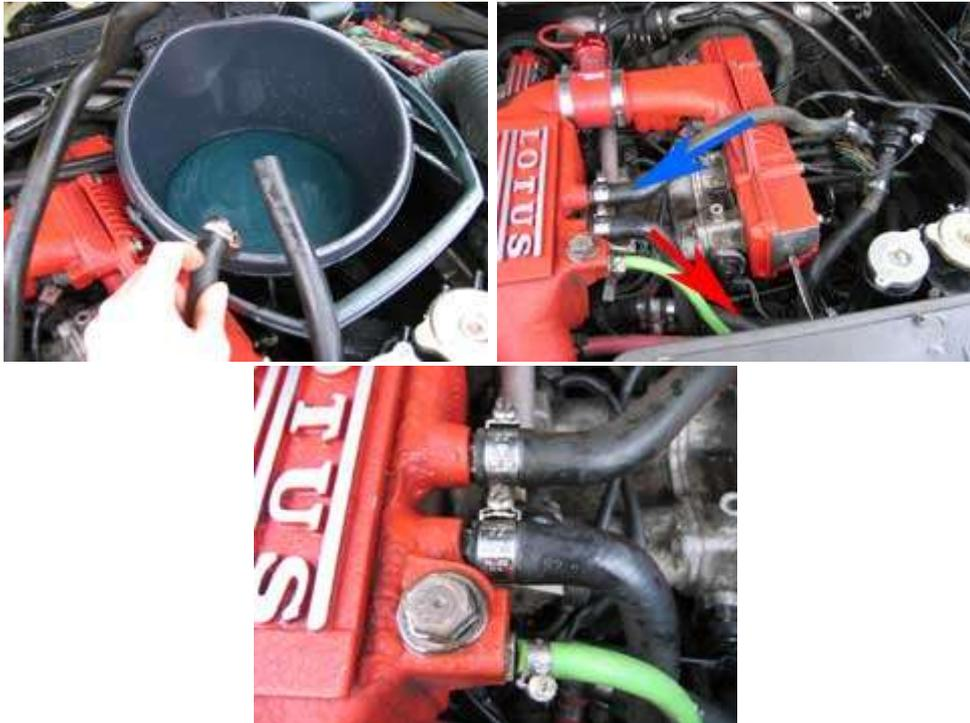
Take the top plug out of the CC and top up, run the pump topping up the CC and there you have it. You can now connect the switch wire that you had connected directly to the battery up to the correct wires to complete the system.
